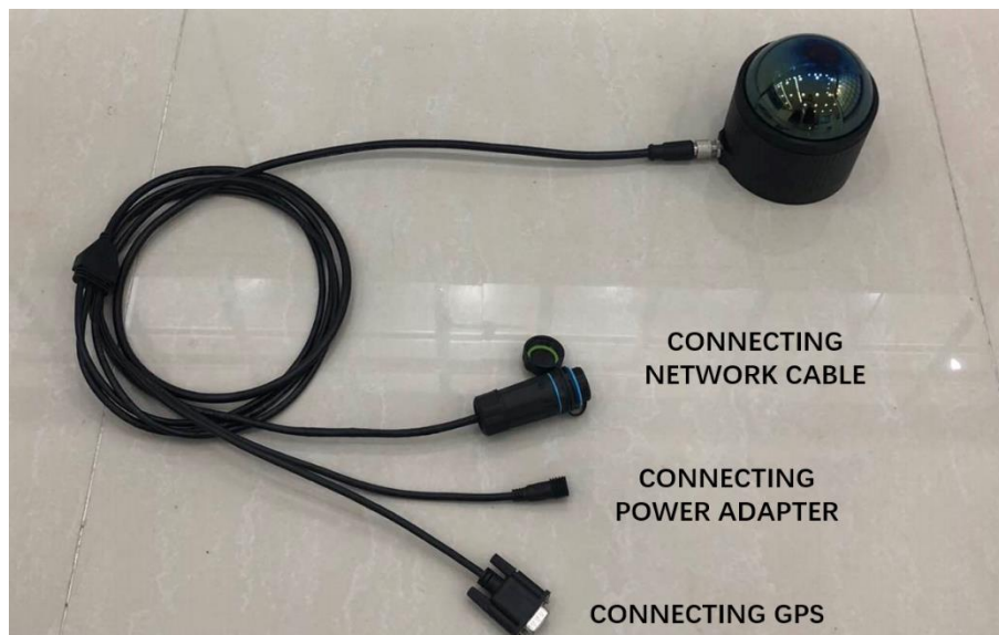
Figure 3.1 Connecting Lidar and Computer
